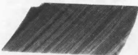
E. Laminated cherty hematitic metatuff (tetsusekiei) that stratigraphically overlies the deposit along its eastern flank. The light laminae are the tuffaceous (sericite-rich) component whereas the darker laminae represent the exhalative (quartz-hematite) component.
