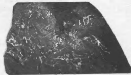
D. Fine chalcopyrite stringer mineralization (light gray) overprinting massive pyritic sulfide, copper zone.
