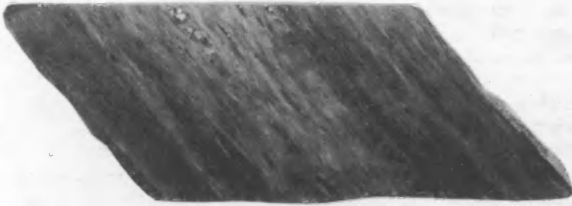
A. Altered felsic quartz-crystal metatuff (quartz-sericite schist) host rock, productive XT unit. Note flattened and elongated blue (dark gray in photo) quartz eyes which characterize this unit.
