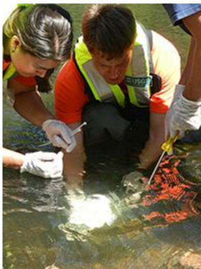
USGS scientists deploy SPMD and POCIS samplers to collect waterborne contaminants in Manoa Stream on Oahu, Hawaii .
