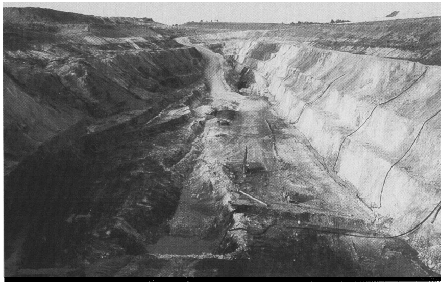
The Flambeau mine near Ladysmith, Wisc., looking northeast with the hanging wall to the left and the footwall to the right.
